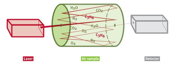
cules – in this case acetone molecules. Lower light intensity on the detector thus indicates a higher acetone concentration in the investigated air sample. This method has the advantage of dispensing with the need for the time-consuming preparation of samples in the laboratory and can produce the measurements within minutes.
